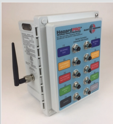
External Whip attached to side of Node
