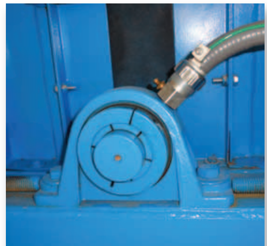
TT420Z-LT installed in a pillow-block bearing.
